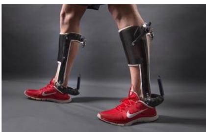
Walking with a passive-elastic ankle exoskeleton. An unpowered clutch engages a spring in parallel with the Achilles tendon when the foot is on the ground, offloading the calf muscles and making walking easier.
